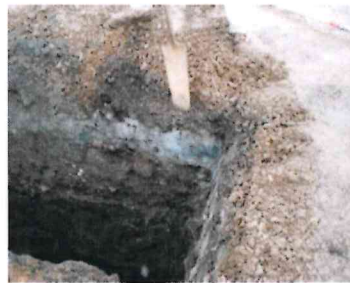
TP- 2 profile: Fine slag/foundry sand layer followed by and MGP purifier waste layer, followed by a rocky slag layer
