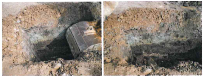
TP- 8 profile: mostly rocky, cemented slag with a layer of MGP purifier waste
